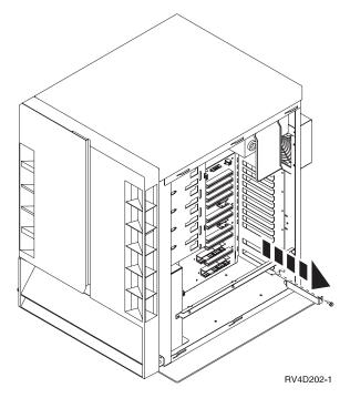
Figure 5. Remove Slot Cover
